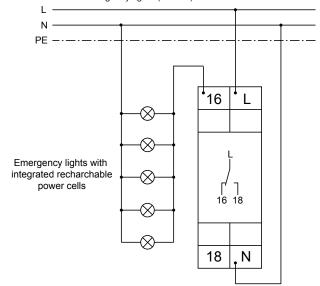
Switching emergency lights with contactor (I > 16A)
