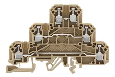
Three-level initiator terminal | Multi-wire terminal, Screw connection, Mounting type:Mounting rail TS 35/7.5 and TS 32, Rated cross-section: 2.5 mm<sup>2</sup>, Width: 5 mm, Colour: Beige
