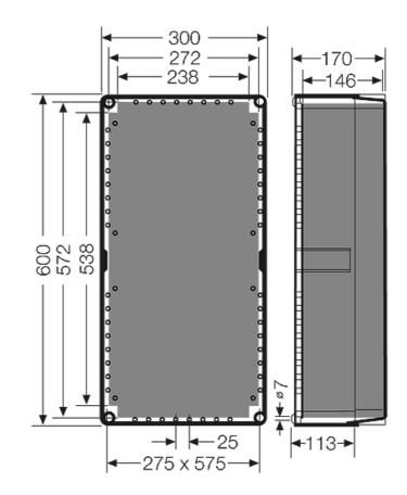
2xM20,10xM25 -1xM32/40 8xM32 8xM32 4xM40/50 4xM40/50 -4xM25 3xM40/50
