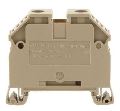
Feed-through terminal, Screw connection, Mounting type: Mounting rail TS 35/7.5, Rated cross-section: 16 mm², Width: 12 mm, Colour: Beige
