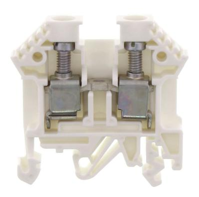
Feed-through terminal, Screw connection, Mounting type:Mounting rail TS 35/7.5 and TS 32, Rated cross-section: 10 mm², Width: 8 mm, Colour: White
